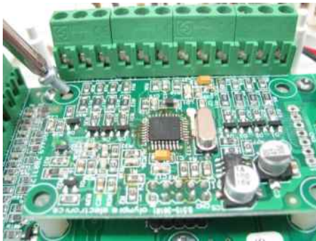
Figure 5 : installing the screws on the BS-469 board.
