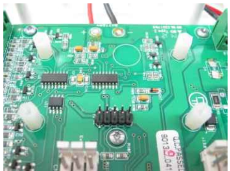
Figure 3 : All spacers fitted.
